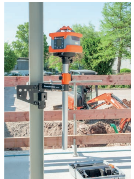
Attachment to a steel beam with a screw clamp
