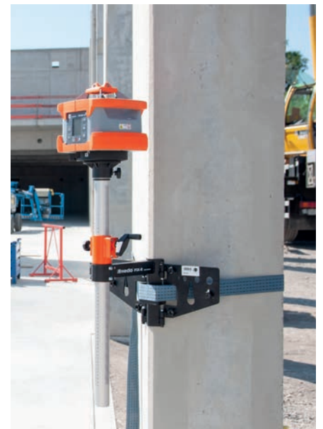
Attachment to a concrete pillar with a tension strap
