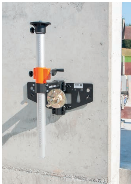
Attachment to a wall with a tie rod
