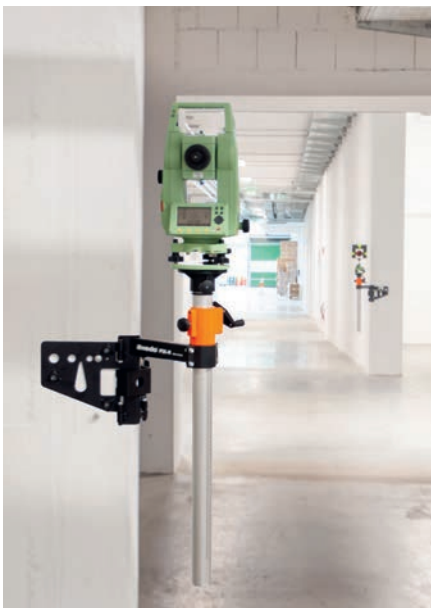
Attachment to a wall with screws
