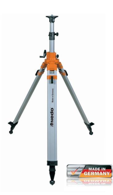
210 678-185 Ref.-No. Min. effective height approx. 40" / 1.01 m Max. effective height approx. 116" / 2.94 m approx. 52" / 1.32 m Retracted length Weight approx. 7.44 kg Tripod plate, Ø 4.3" / 110 mm Holding screw 5/8" x 11 thread **Telescopic section** 2-fold Adjustable column range 20"/19" / 490/520 mm
