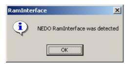
The software is ready to work after pressing 'OK'. If the matching serial port is not selected, Nedo Connect XP<sup>®</sup> will not be able to communicate with the Nedo interface.
