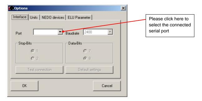
Please select the serial port by clicking on the drop down list. All other parameters need not to be adjusted, if the interface is still set to default (factory) settings (2400,n,8,1).
