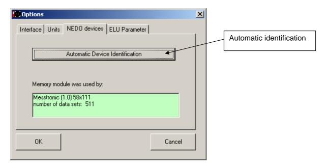
The example above shows a memory module that was used with a mEsstronic 583111, and there are 511 datasets in the memory module's memory.
