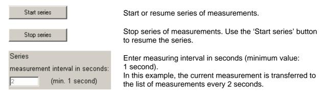
**Caution:** When taking measurements over a long period, do not define a too short measuring interval, as otherwise a large amount of measurement data will be generated that requires a correspondingly large amount of PC memory.
