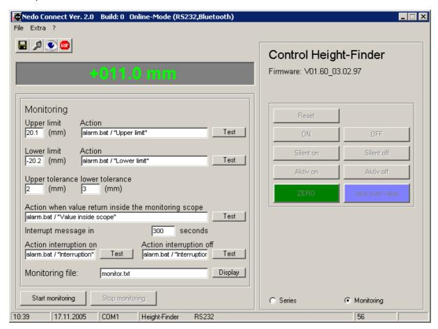
If the measurement received exceeds the upper limit of 20.1 mm, the program *alarm.bat* is executed with the parameter "Upper limit".
