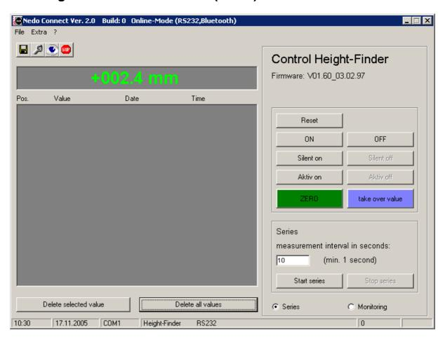
The Height-Finder user interface provides a very wide range of functions, and is divided into three function blocks:
