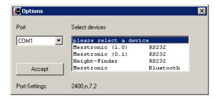
The appropriate interface parameters are automatically set by the program. Confirm selection with the 'Accept' button.
